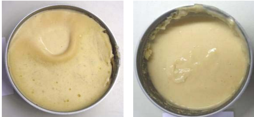
Figure 6.13: Solidification of egg batter in Ø 127 metal container after 130 s in the Panasonic oven.
