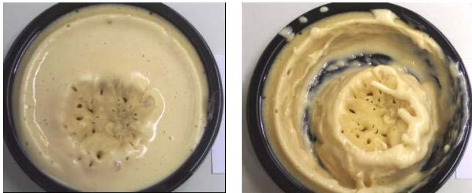
Figure 6.16: Solidification of egg batter in \varnothing 127^* plastic container after 86 s in the Micromaxx oven.
